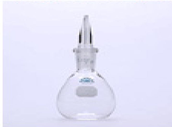
Specific gravity bottle, picnometer (Gay-Lussac style)
