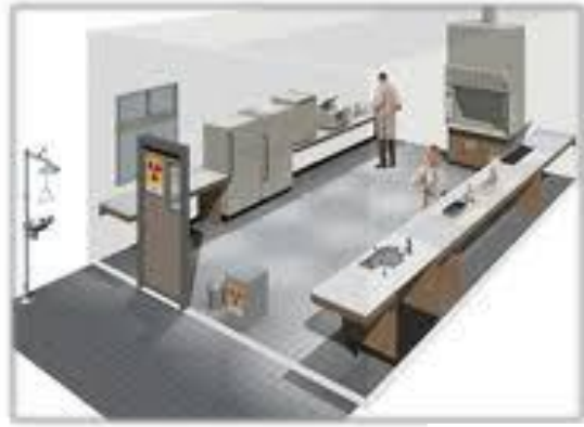
Figure 1. A typical BSL-1 laboratory. MTC, Inc., 2014. Copyright © MTC, Inc. All rights reserved.
